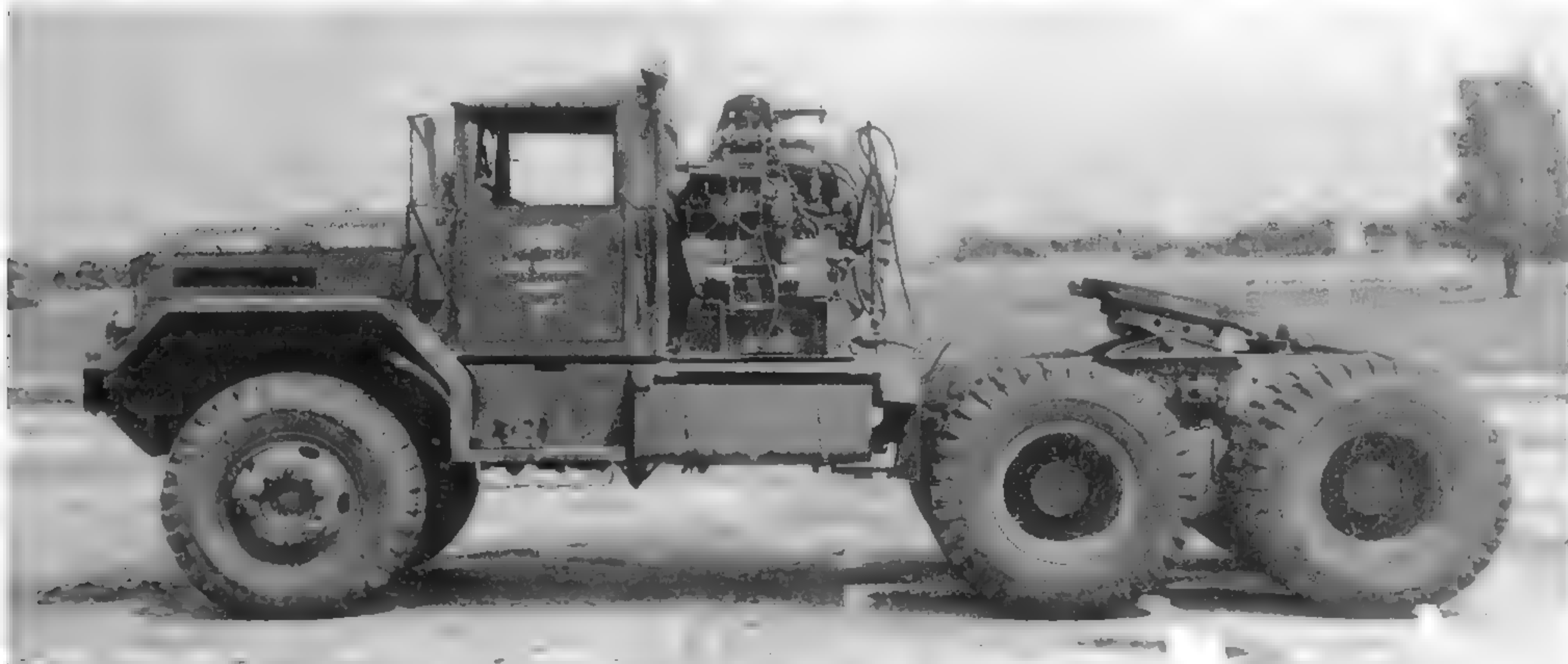
The M123A1C was factory built as a diesel-powered truck. Some diesels, like this vehicle photographed at Aberdeen Proving Ground, had dual horizontal exhausts, as did the gasoline-powered trucks. Others had a single vertical exhaust stack. (U.S. Army photo)
